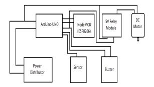
Fig. 3. Circuit representation of the prototype
