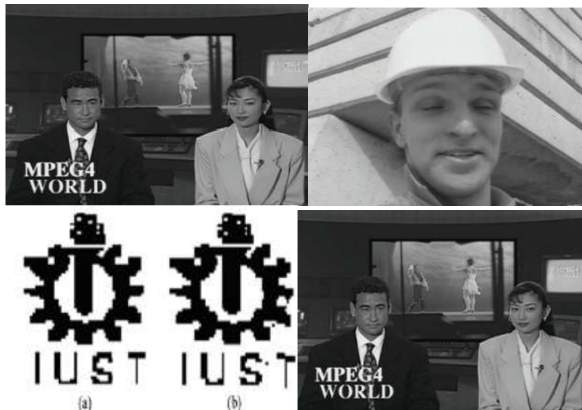
Figure 3. a) The original 100 frame sequence. b) 100 frame sequence original image. c) Extracted and original watermark with NC = 0.9929. d) Watermarked video. (PSNR = ~ 40)
