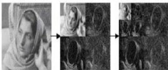
Fig 4: a picture is isolated into different diverse sub bands. The LL sub band is additionally decayed into four other sub-bands. The LL sub band holds greatest data.
