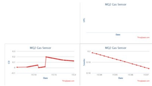
Fig.6. Air pollution monitoring using MQ2.
