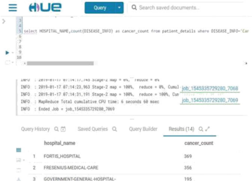
Fig. 8 Query without partition in Hive: number of cancer patients visited to hospital
