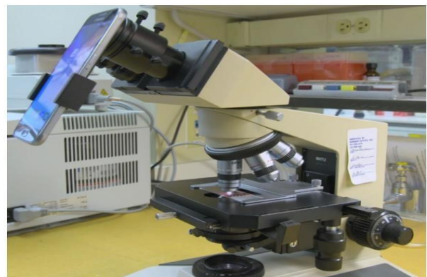
Fig.1: Malaria data acquisition via smartphone
