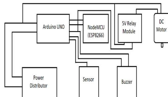
**Fig. 3.** Circuit representation of the prototype
