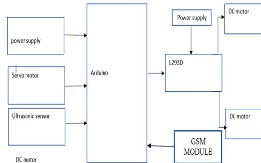
Fig.2: System architecture
