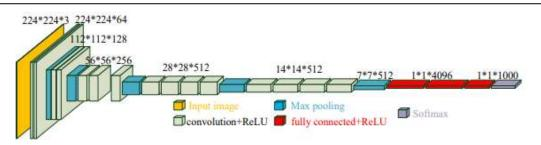
Fig.,-3 VGG-19 Net CNN model
