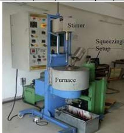
**Fig. 1.** Squeeze casting setup for MMC processing
