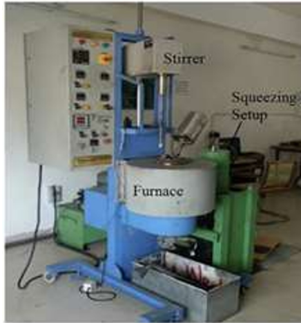
Fig. 1. Squeeze casting setup for MMC processing.
