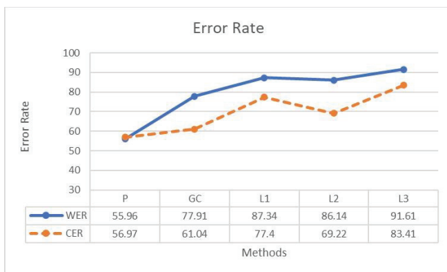
Fig. 6. Graph representing Methods vs Error Rates (Word, Character) (where P represents Direct prediction (without auto-correct), GC represents Ratcliff/Obershelp algorithm, L1-L2-L3 represent Leveshtien1-Levenshtien2-Levenshtien3 respectively)
