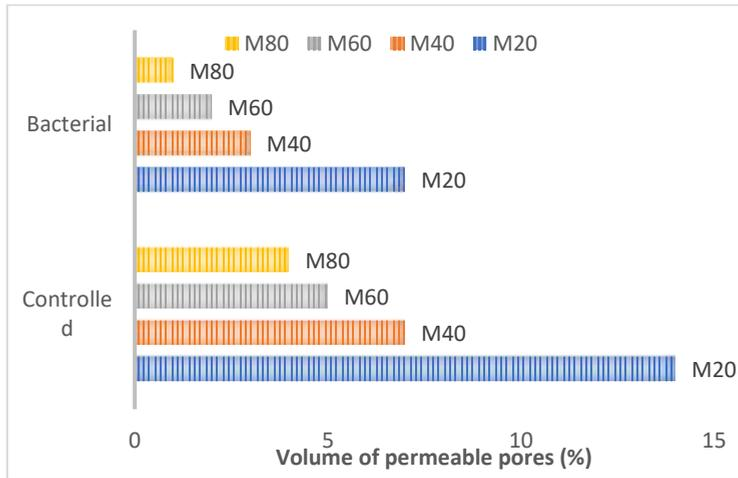
**Fig. 3.** Water absorption Capacity and volume of permeable pore space of controlled and bacterial concrete
