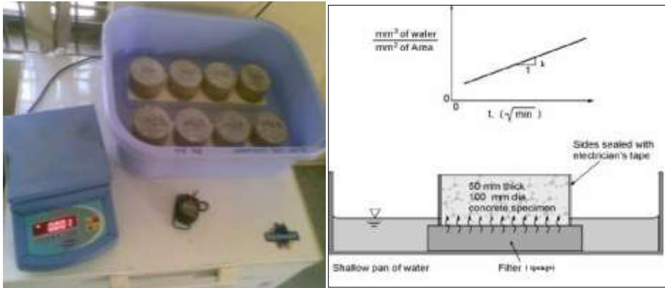
**Fig 1.** Experimental Setup for Sorptivity Test
