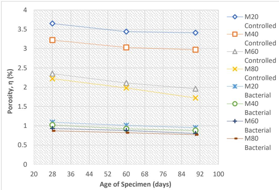
**Fig. 6.** Variation of porosity with age for different grades of reference and bacterial specimens
