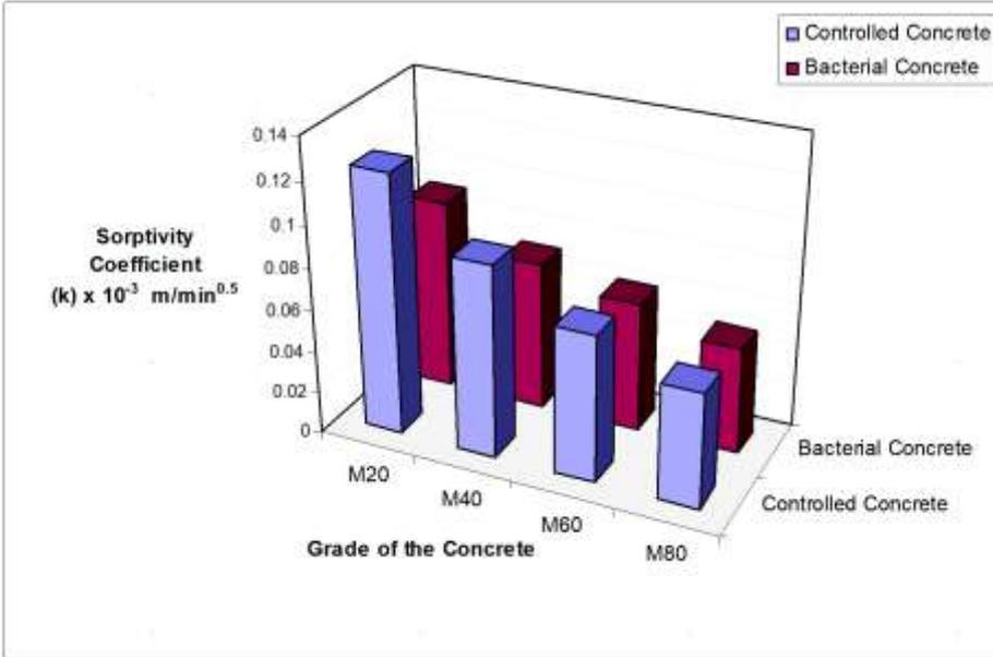
**Fig. 5.** Variation of sorptivity of reference and bacterial specimens for different grades
