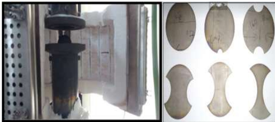
Fig. 2. Sheet Metal Forming setup & One set of specimens used for plotting the FLD
